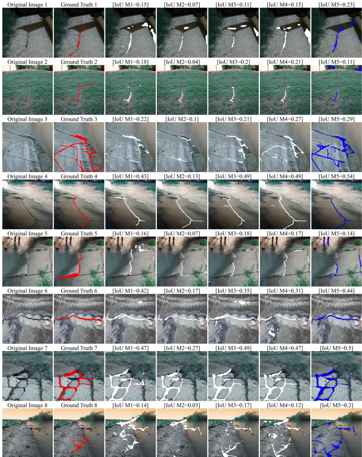
FIGURE 4. Examples from the independent levee crack test dataset from Experiment 1. Each colored column above represents a mask overlaid on the original image. White-colored masks are predicted segmentation masks for U-Net (M1), MultiResUnet (M2), Attention U-Net (M3), and UNet++ (M4). The red-colored mask is the ground truth, and the blue mask is the predicted segmentation mask by IterLUNet (M5).
